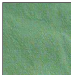
Fig. 12. Wool fabrics dyed with copper cyclohexane di carboxylate at 6 g/l dye concentration
