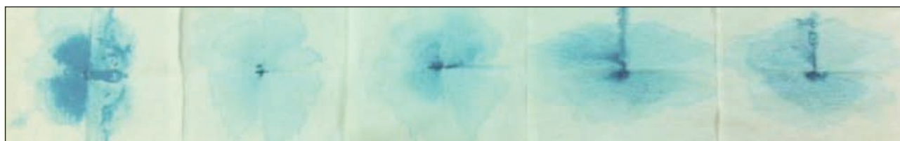
Fig. 3. Images of filtration sheets of dye solutions prepared in the presence of ultrasound with 5 different dispersing agent concentrations (0.5; 1; 1.5; 2; 2.5 g/l) at 6 g/l copper cyclohexane di carboxylate concentration and pH 7
