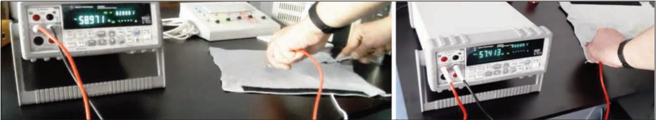
Fig. 2. Determination of the variation of the electric current in the conductive textile electrodes and of the frequency
